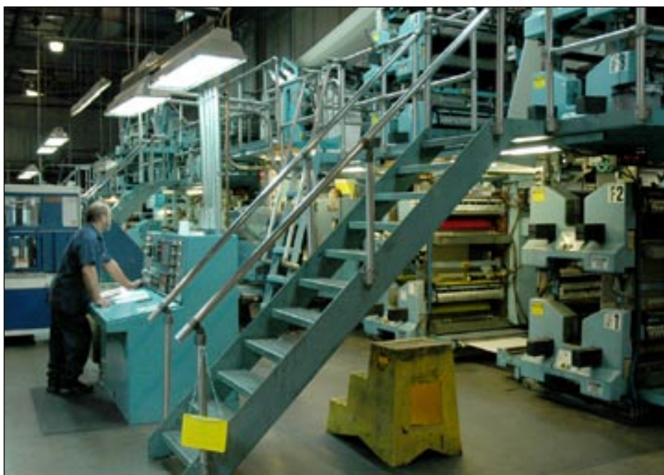
While not small compared to the presses used by many community dailies, this 20-unit DGM 1030 press is significantly smaller than the Tribune ’s main press, the 48-unit Goss Universal 45. These presses allow the Tribune to print many newspapers besides its own.
